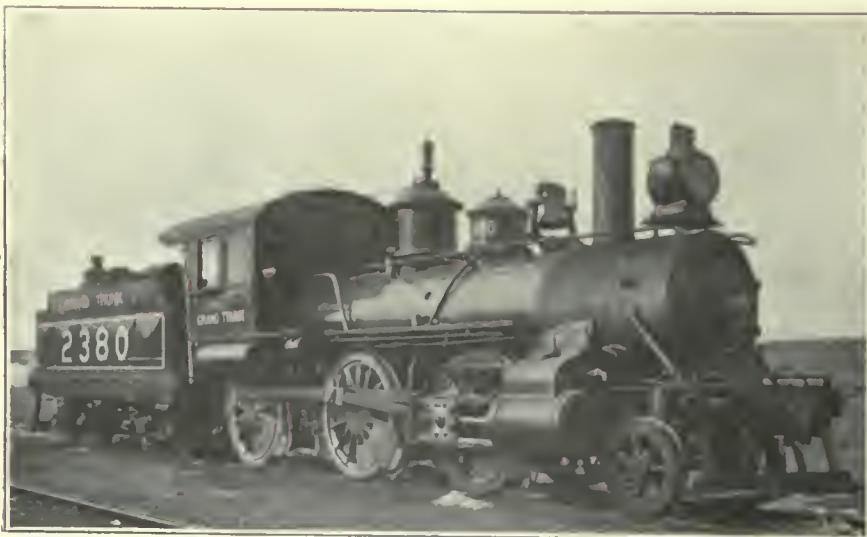
FIG. 386. LOCOMOTIVES. Locomotive of the Mogul Type. An older type of freight loco- motive. Grand Trunk Western Rail- way.
